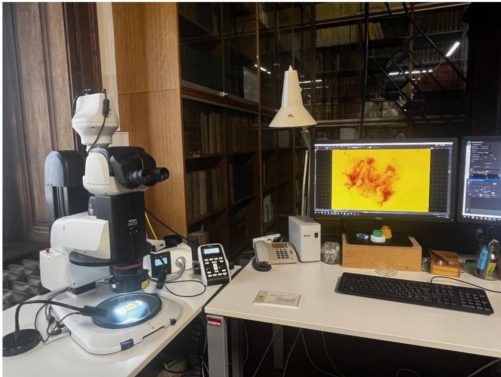
Fig. 6. Nikon DS-Ri2 camera mounted on a Nikon SMZ25 stereomicroscope. Photo credit N. Akkari
